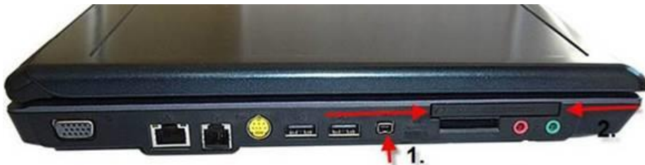
1. IEEE 1394/DV - 4-pin (internal) 2. ExpressCard 34/54 or PCMCIA Card Slot (w/ 6-pin Firewire adaptor card)
